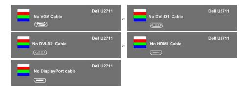
This box also appears during normal system operation if the video cable becomes disconnected or damaged.
